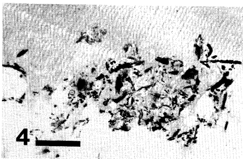
Fig. 4. A transmission electron micrograph of a section taken through a "particle" like the one shown in Fig. 3. Note that the increased resolution of Fig. 4 reveals the "particle" to be a heterogeneous aggregate of colloids, one which includes globules. The bar represents 3 \mu\text{m} .
